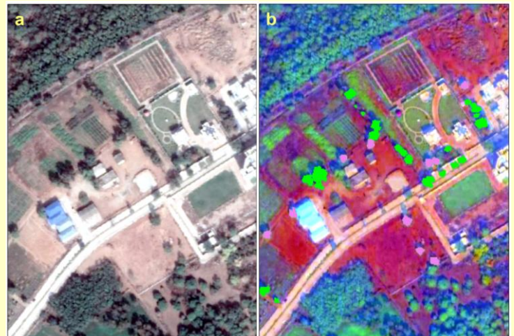
Fig. 1: Instance segmentation using the tree dataset. (a) Initial image in its natural colour (b) PCA image with individually labelled tree crowns.
